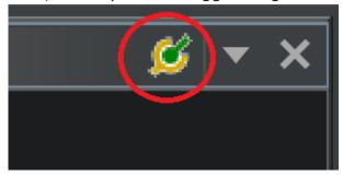
This will open the debugger connector window. In the drop down, select gdb, and as the launch command, enter the path to the gdb multiarch binary, followed by -i mi2. For example, on Windows, this could be
