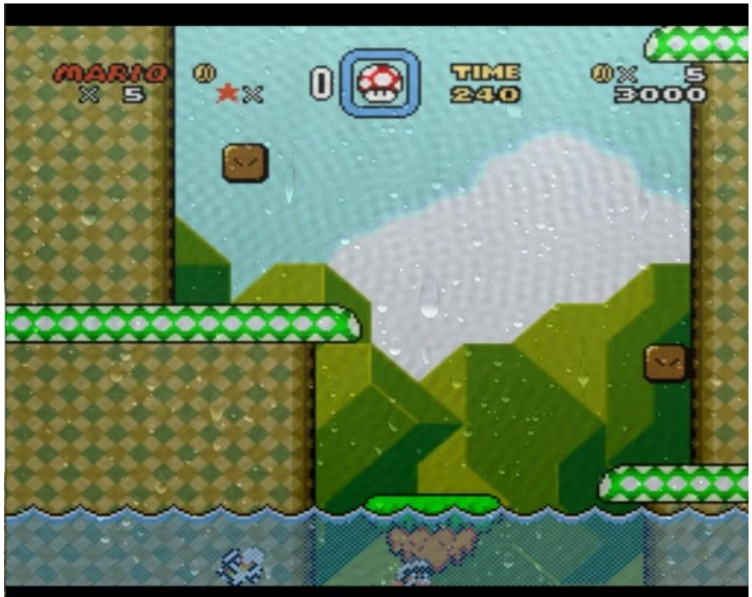
Figure 4: Super Mario World with a game aware shader applying a LUT texture as soon as Mario jumps into the water.
